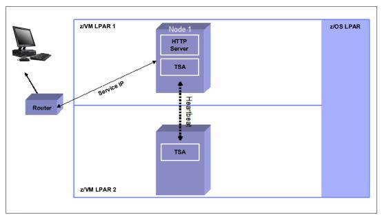
Figure 6-16 Normal situation: Tivoli System Automation monitors for outages
