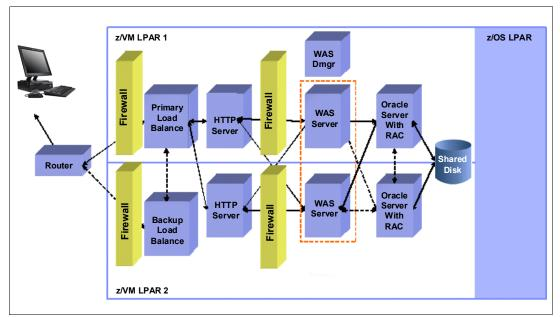
Figure 6-20 Database sharing using Oracle RAC
