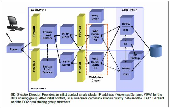
Figure 6-21 Database sharing using z/OS Parallel Sysplex
