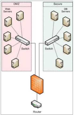
Figure 6-6 Multiple distributed network scenario: DMZ segmented network
