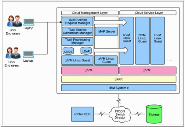
Figure A-1 Cloud solution using Linux on System z
