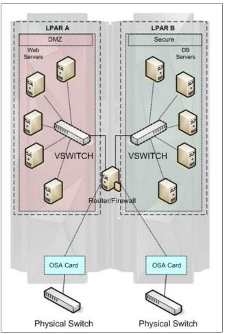
Figure 6-7 Multiple virtualized network scenario: DMZ and secure network
