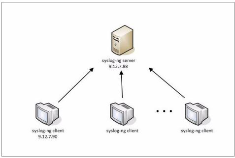
Figure 7-9 A centralized syslog-ng server and some syslog-ng clients
