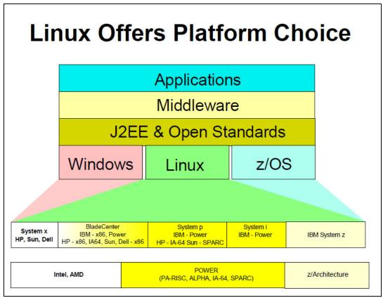
Figure 1-1 Variety of commercial IT platforms supported by Linux
