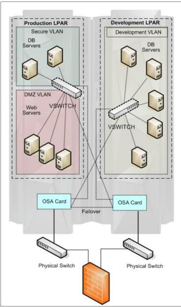
Figure 6-8 Multiple virtualized network scenario with failover: DMZ and secure network
