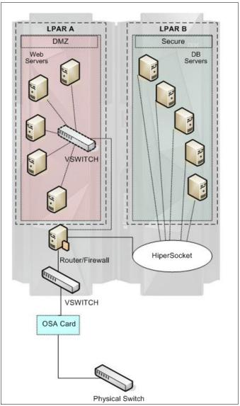
Figure 6-9 Multiple virtualized network scenario with multiples LPARs
