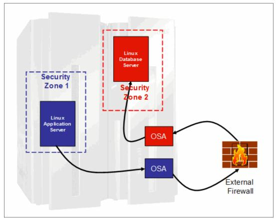
Figure 6-13 Using external firewalls between security zones
