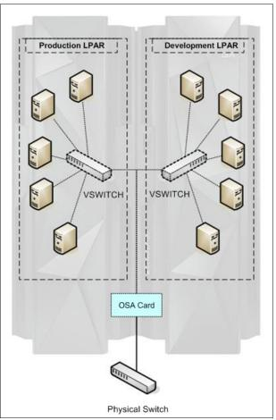
Figure 6-4 Single virtualized network with multiple LPARs
