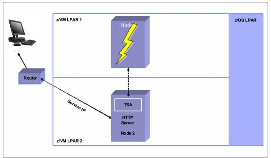
Figure 6-17 Outage occurs: Tivoli System Automation fails over to cold standby
