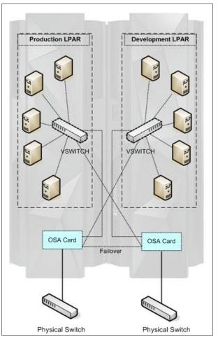
Figure 6-5 Single virtualized network with multiple LPARs and failover
