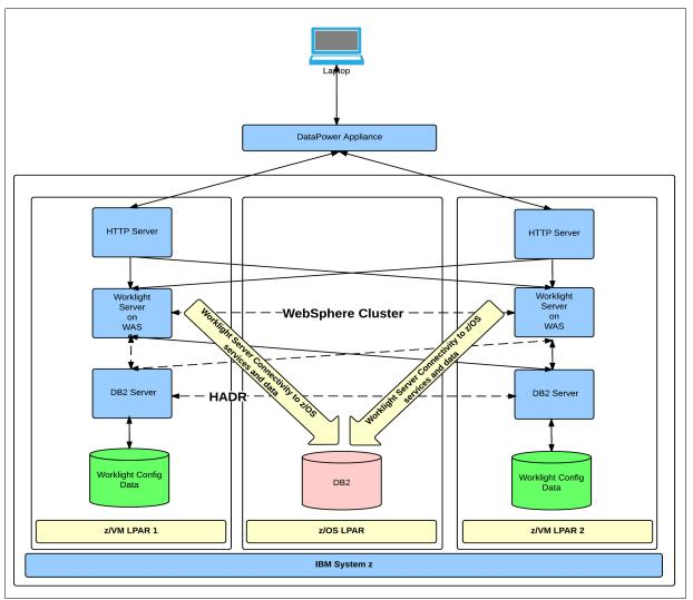
Figure A-2 Access from a mobile device to a back-end transactional core system
